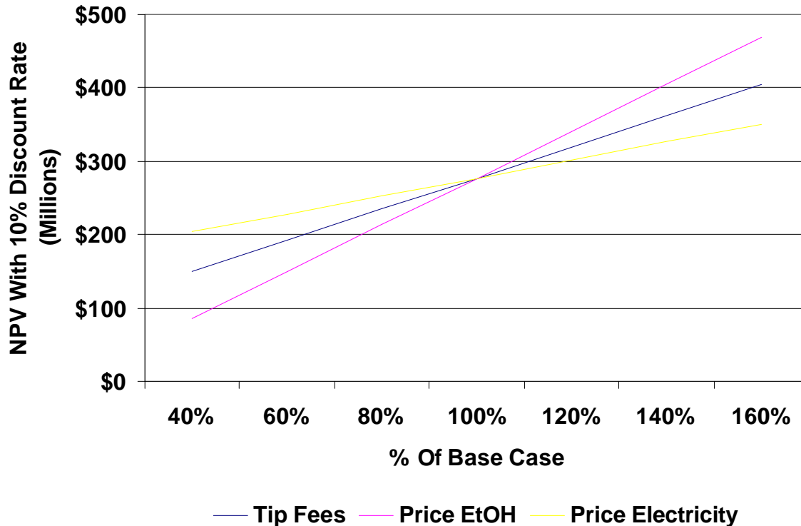
Figure 1. Net present value of a 3000 TPD MSW-based biorefinery with a 10 % discount rate. This economic model forecasts a process with no additional pretreatment (41 % hydrolysis rate).
