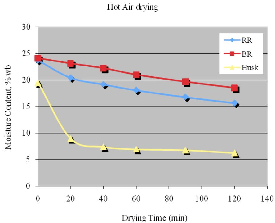
Figure 17: Changes in Moisture content of Rough rice, Brown Rice and Husk during continuous hot air drying
