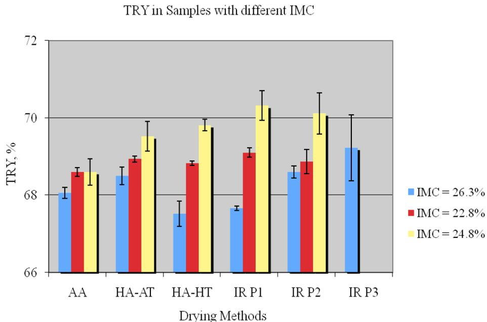
Figure 5: Total Rice Yield (TRY) in different drying methods. IMC: Initial moisture content on wet basis, AA: Ambient Air drying, HA: Hot Air drying, AT: Ambient temperature tempering, HT: Heated temperature tempering, IR: Infrared drying, P1: one pass, P2: two passes and P3: three passes
