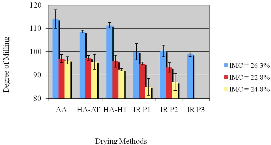
Figure 7: Degree of milling (WI) in different drying methods.
