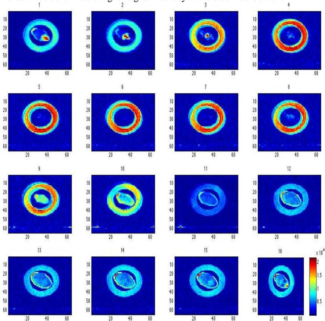
Figure 14: MRI Signal intensity of sixteen slices along the transverse plane at start of drying
