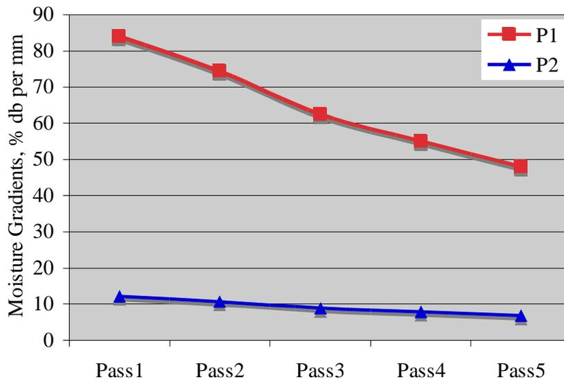
Figure 11: Moisture content gradients at bran-husk interface (P1) and at bran-endosperm interface (P2) after each pass in the hot air drying process
