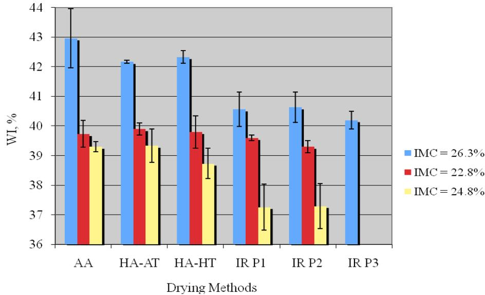
Figure 6: Whiteness Index (WI) in different drying methods. IMC: Initial moisture content on wet basis, AA: Ambient Air drying, HA: Hot Air drying, AT: Ambient temperature tempering, HT: Heated temperature tempering, IR: Infrared drying, P1: one pass, P2: two pass and P3: three passes
