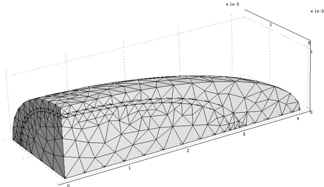
Figure 1: Three dimensional model of rice kernel in Comsol Multiphysics simulation program
