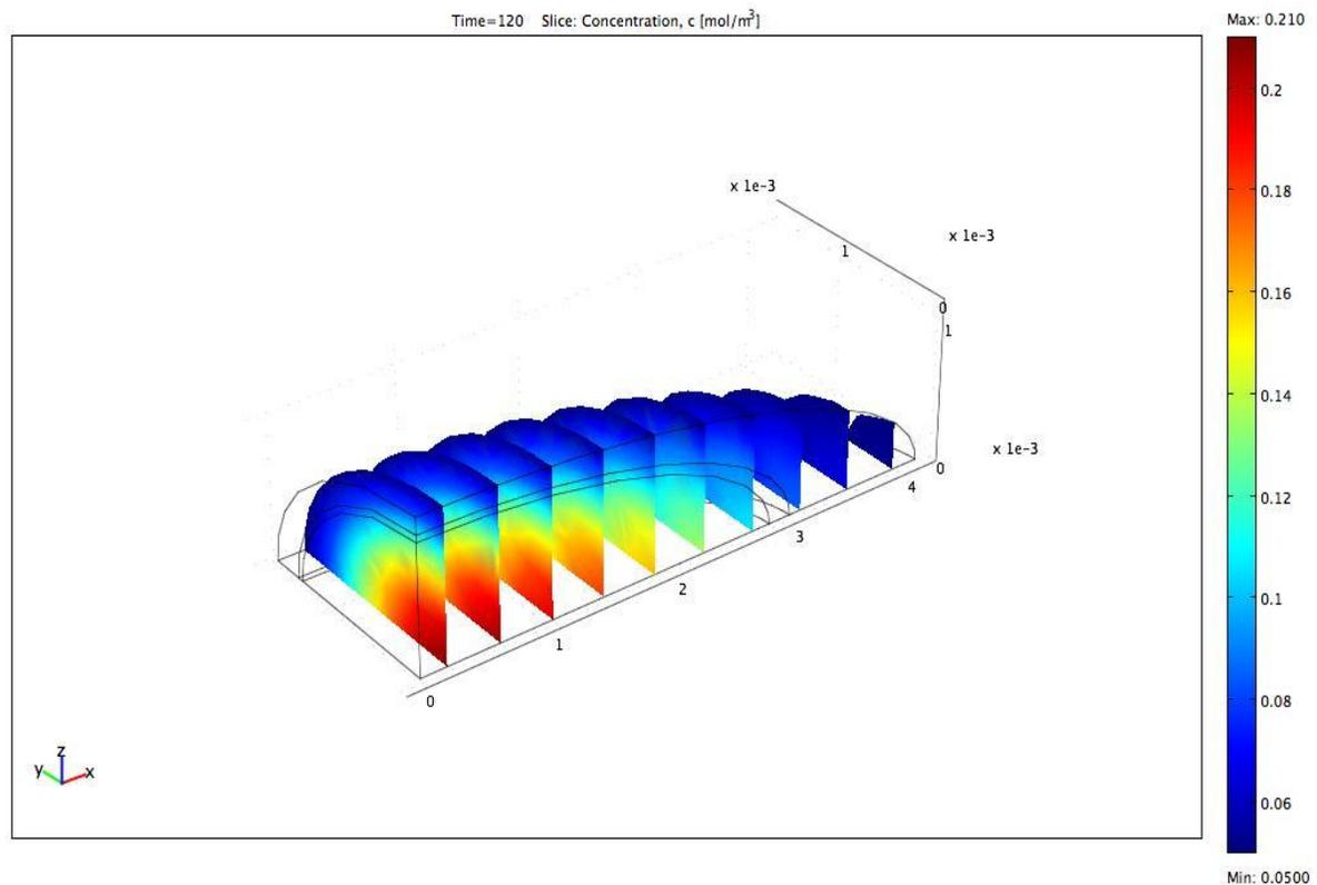
Figure 8: Moisture content ( fraction, d.b.) in rice after two hours of ambient air drying.
