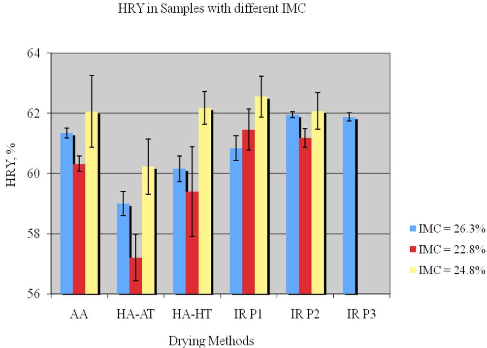
Figure 4: Head Rice Yield (HRV) in different drying methods. IMC: Initial moisture content on wet basis, AA: Ambient Air drying, HA: Hot Air drying, AT: Ambient temperature tempering, HT: Heated temperature Tempering, IR: Infrared drying, P1: one pass, P2: two passes and P3: three passes
