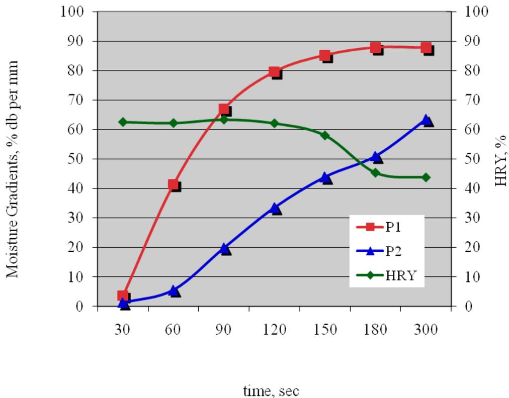
Figure 12: Moisture content gradients at bran-husk interface (P1) and at bran-endosperm interface (P2) during infrared drying process and Head Rice Yield obtained in the experiments conducted in same conditions.
