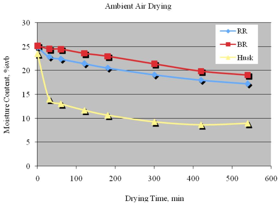
Figure 16: Changes in Moisture content of Rough rice, Brown Rice and Husk during continuous ambient air drying
