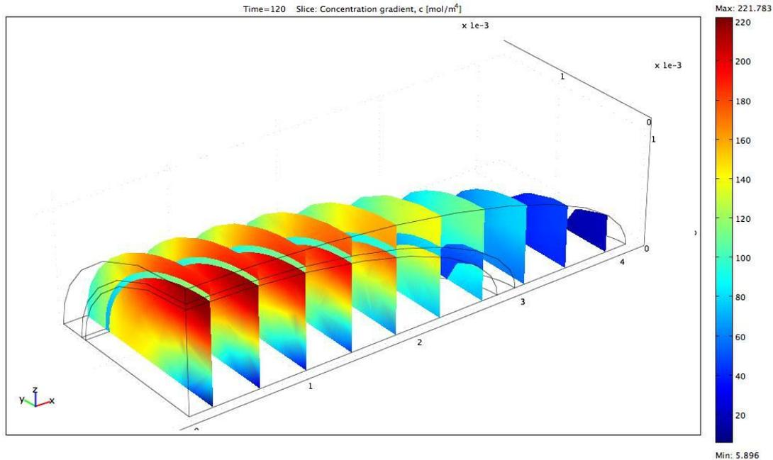
Figure 9: Moisture content gradient (d.b.) in rice after two hours of ambient air drying
