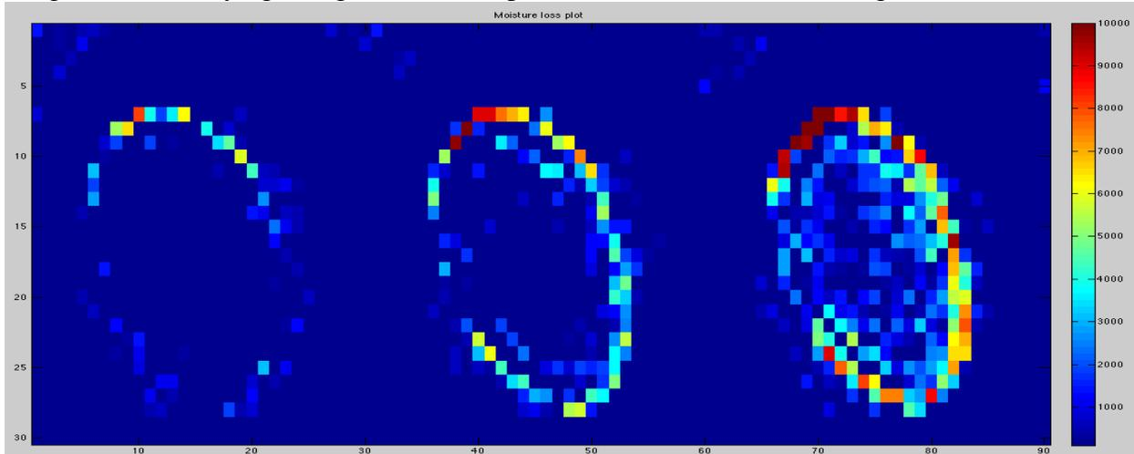
Figure 15: Subtraction plots of center slices in first, second and the third hour of drying
