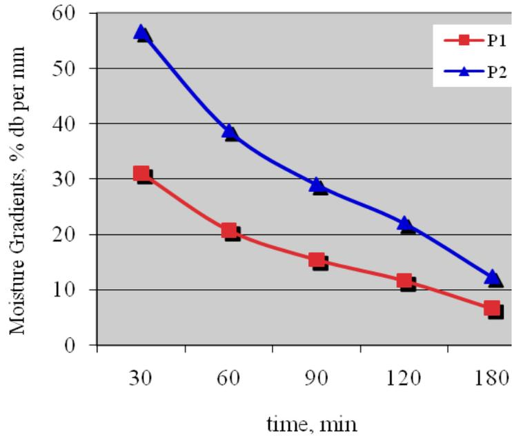
Figure 10: Moisture content gradients at bran-husk interface (P1) and at bran-endosperm interface (P2) during continuous ambient air drying process
