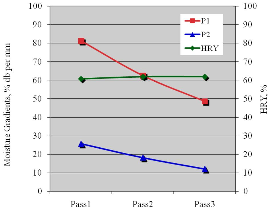
Figure 13: Moisture content gradients at bran-husk interface (P1) and at bran-endosperm interface (P2) after each pass and corresponding Head Rice Yield in the infrared drying process
