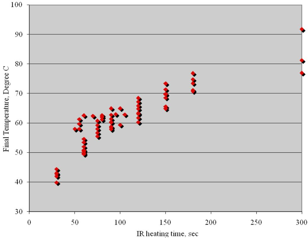
Figure 3: Final surface temperature reached during infrared heating of rough rice having different initial moisture contents at IR intensity of about  $4000 \text{ W/m}^2$
